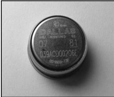
The upgrade key is a small hardware device installed in the SVMi-4E daughter board card. It provides the license for two additional ports increasing the number of available ports from 2 to 4, and the number of mailboxes from 25 to 100.
