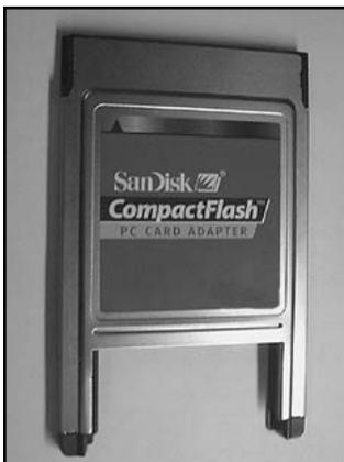
The Back Up Adapter allows the removable memory card to be installed in the PCMCIA card slot of a Laptop PC. When this is done a back up may be made of the customer database. This item is available from [www.sandisk.com](http://www.sandisk.com) or Insight Direct.
